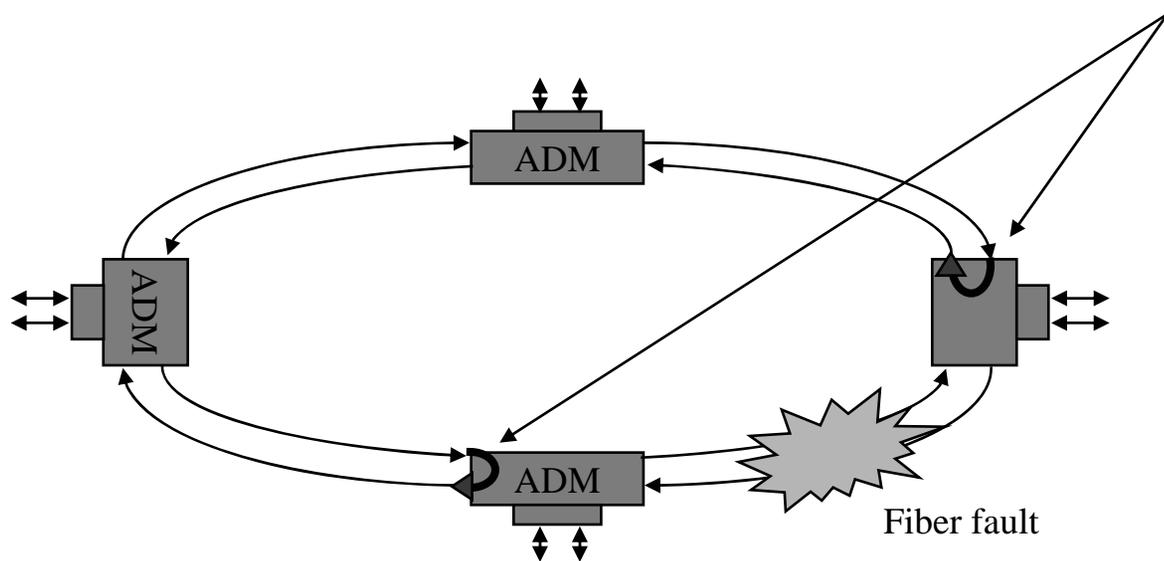
Nodes close to the fiber fault create a loopback to reconfigure the ring
