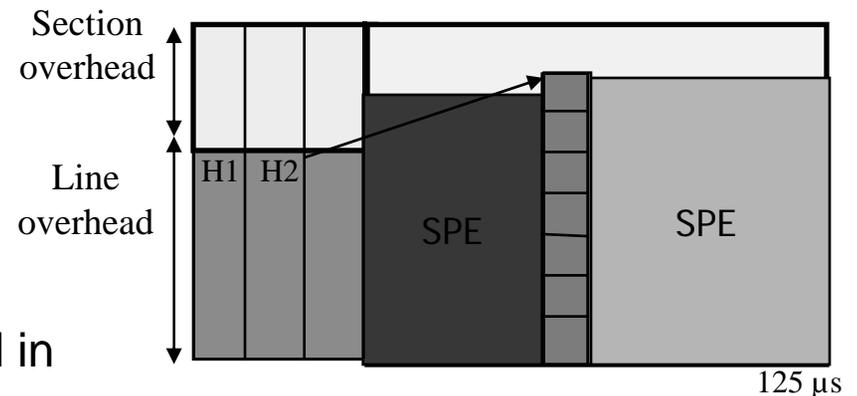
Bit Stuffing was used in PDH. Byte stuffing is used in SONET
