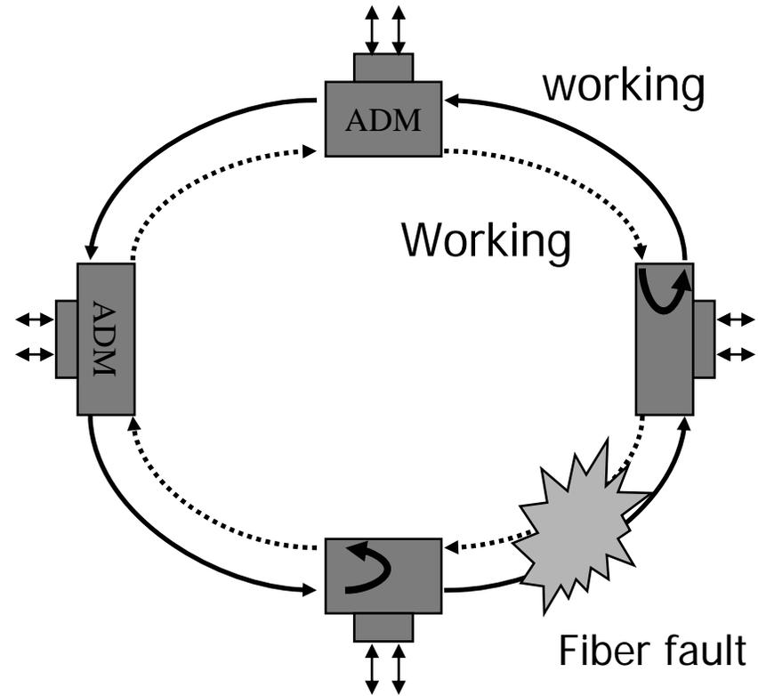
Only nodes close to the fault are involved in the protection
