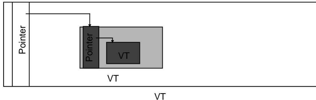
This allows to multiplex contributing tributaries running at very different speed in an efficient manner.
