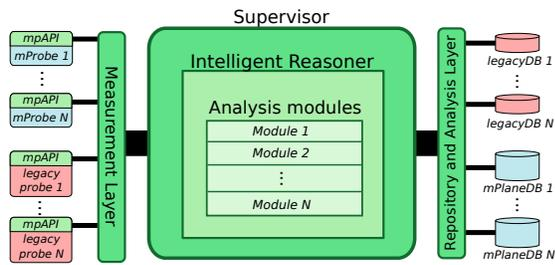
Fig. 7. Schematical representation of the mPlane architecture.
